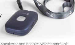
and a built-in speakerphone enables voice communication with the centre's trained staff. GPS, Wi-Fi and beacon positioning all cooperate to provide not only the user's location, but also advanced tracking and geofencing functionality that incorporates energy-saving technology for achieving long battery time.
